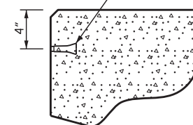
THREADED INSERT DETAIL
